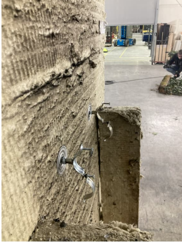
Figure 56: Hook Supports for the Samples
