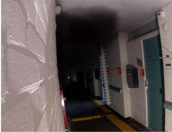
Validation of multizone models for internal smoke propagation (TU/e) by experiments (IFV/Dutch Fire Service Academy)
