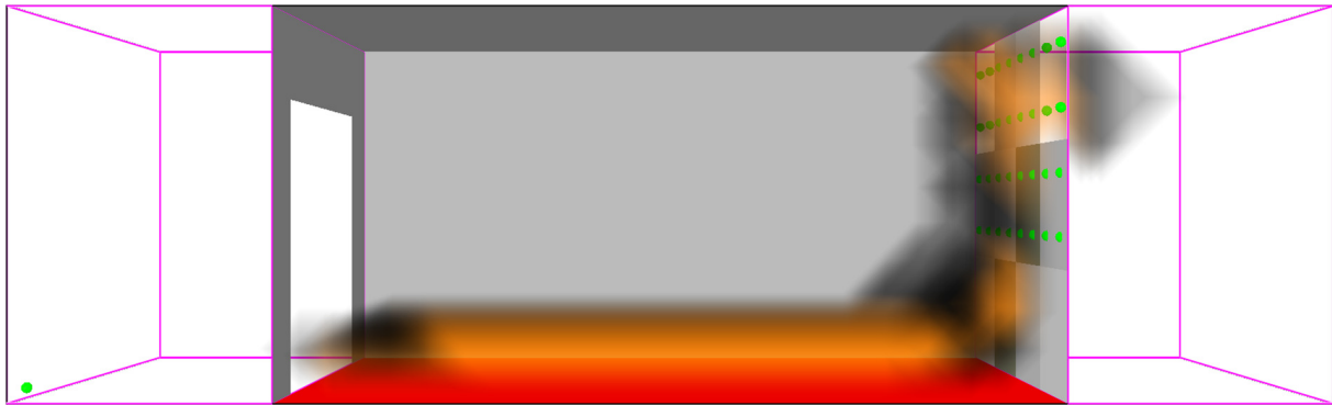
Figure 8.6 – Smokeview visualization of the two-way coupled CFD-FEM simulation @ 865 s.
