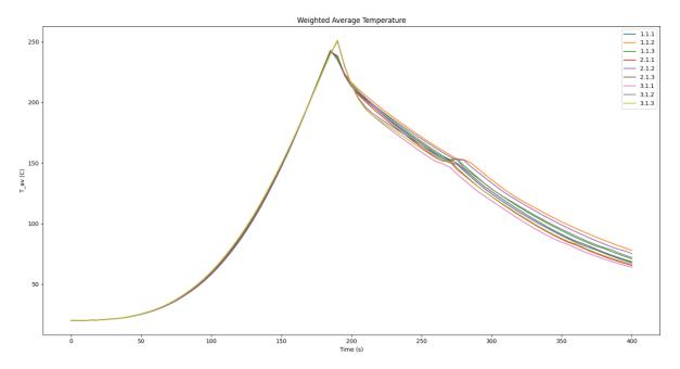
Figure 5-9. Weighted average temperature for all fire scenarios with a medium fire growth rate
