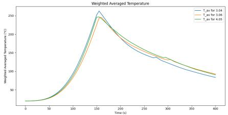
Figure 6-13.  $T_{av}$  curve of the fire scenarios where  $t_a = 150 \text{ s}$
