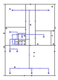
Figure 6-8. CONTAM geometry of apartment 4/A2 without (left) and with (right) modelled bypass
