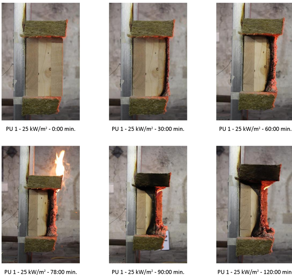
Figure 40. Time-lapse PU 1. 25 kW/m 2 for 120 min. Re-ignition at minute 76.
