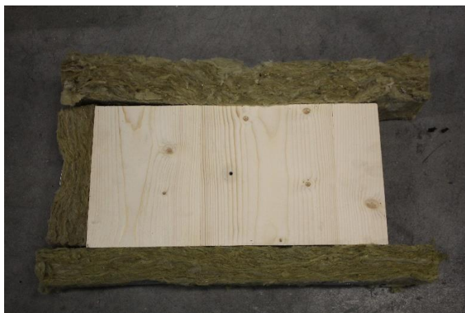
Figure 22. ME - CLT Specimen. X80/3s: 200 mm x 400 mm with lamella of 30 mm, 20 mm and 30 mm.
