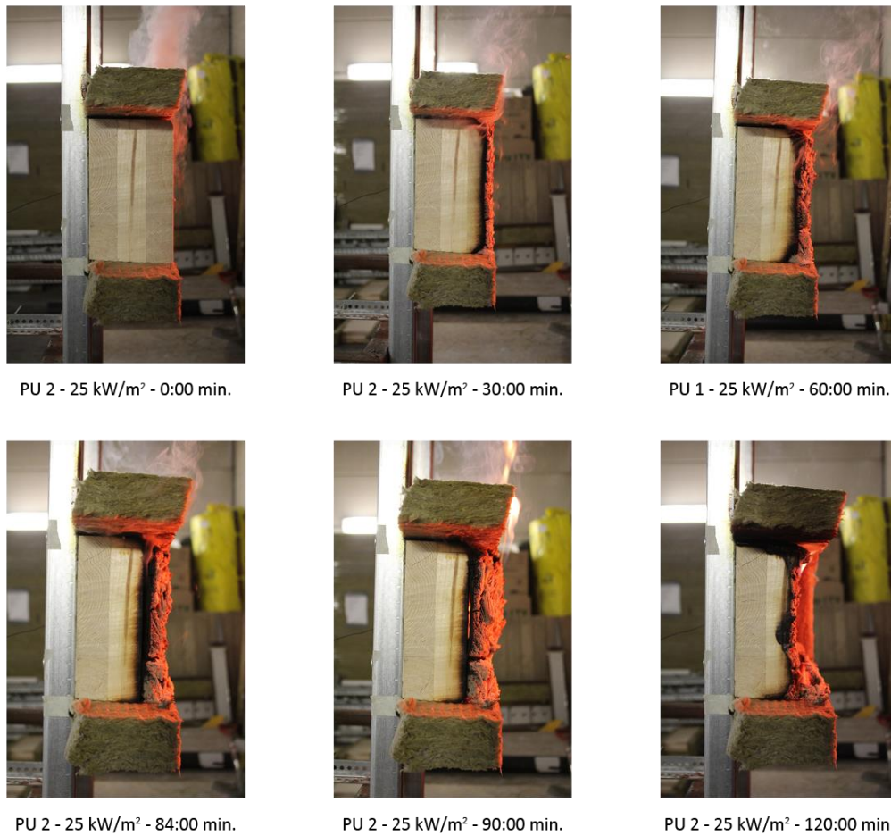
Figure 43. Time-lapse PU 2. 25 kW/m 2 for 120 min. Re-ignition at minute 88.
