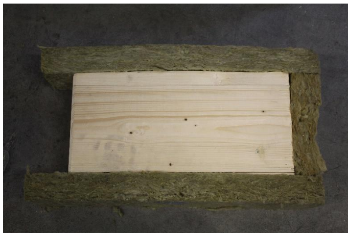
Figure 21. PU - CLT Specimen. L120/3s: 200 mm x 400 mm with lamella of 40 mm (x3).
