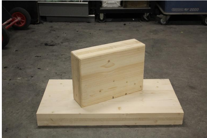
Figure 16. Derix CLT Sample. L120/3s: 300 mm x 400 mm with lamellae of 40 mm (x3).
