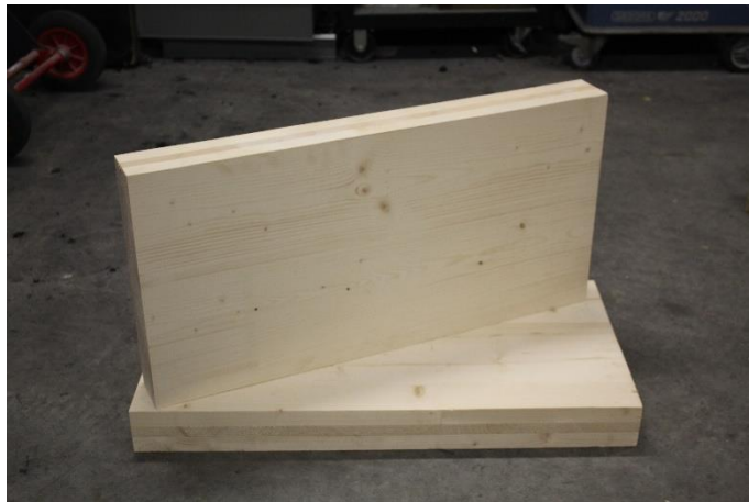
Figure 17. Derix CLT Sample. X80/3s: 400 mm x 800 mm with lamellae of 30 mm, 20 mm and 30 mm.
