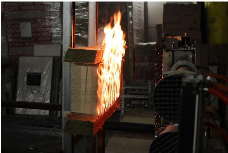
Figure 10. CLT flaming combustion.
