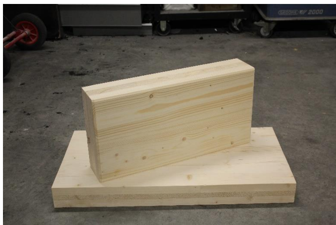
Figure 15. Derix CLT Sample. L120/3s: 300 mm x 600 mm with lamellae of 40 mm (x3).
