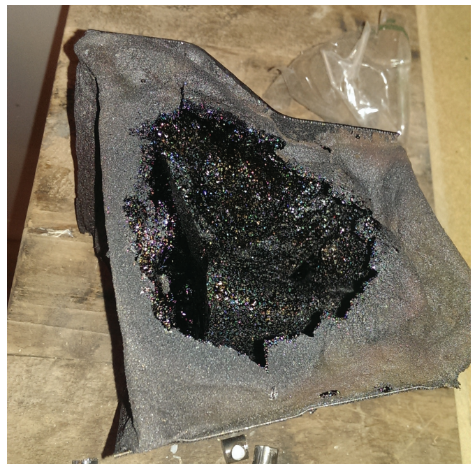
Figure 22 PUR sample after a test
