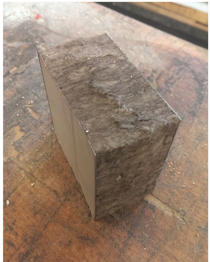
Figure 46 - Discolouration of a SWP sample after a test limits could be established.
