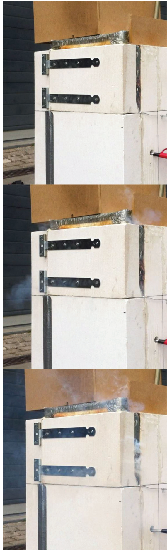
Figure 58 - Stills from a video capturing a smoke gas explosion
