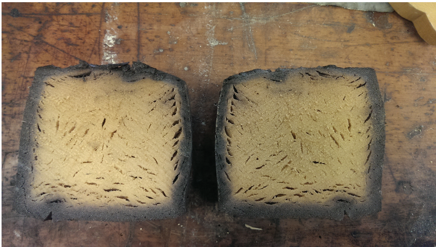
Figure 34 - Section of a PIR sample after a test
