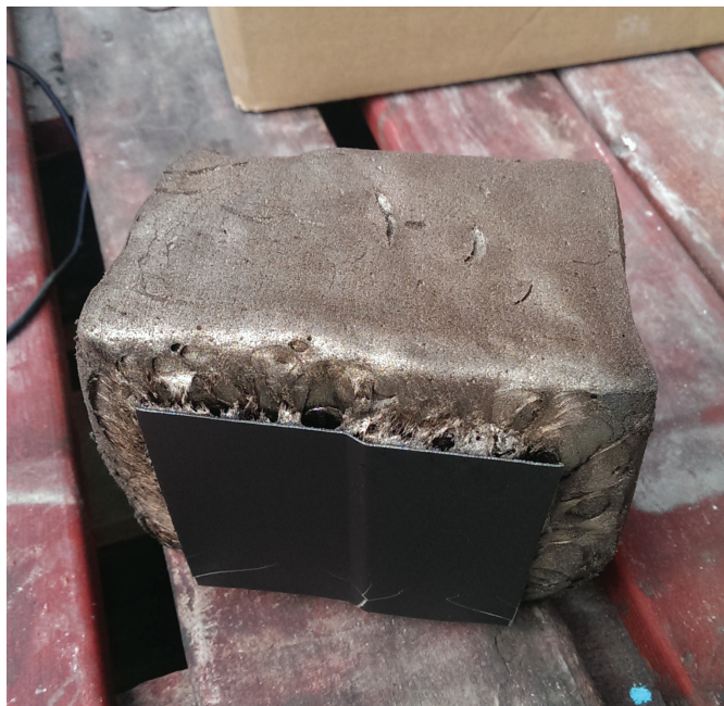
Figure 35 - PIR sample after a test
