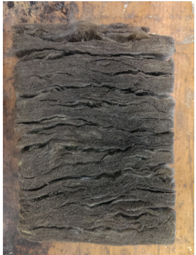
Figure 45 - loose fibres of the SWC after a test
