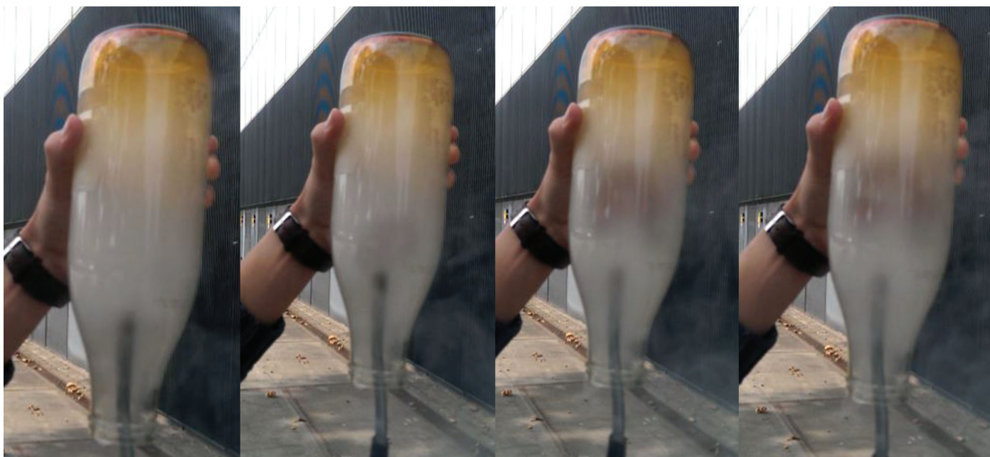
Figure 25 - Stills of a film where smoke is burnt close to a stoichiometric ratio tests.
