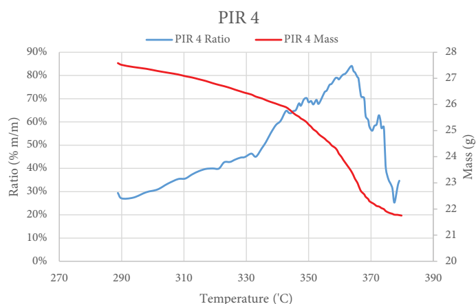
Figure 30 - PIR test 4 mass loss and ratio versus temperature
