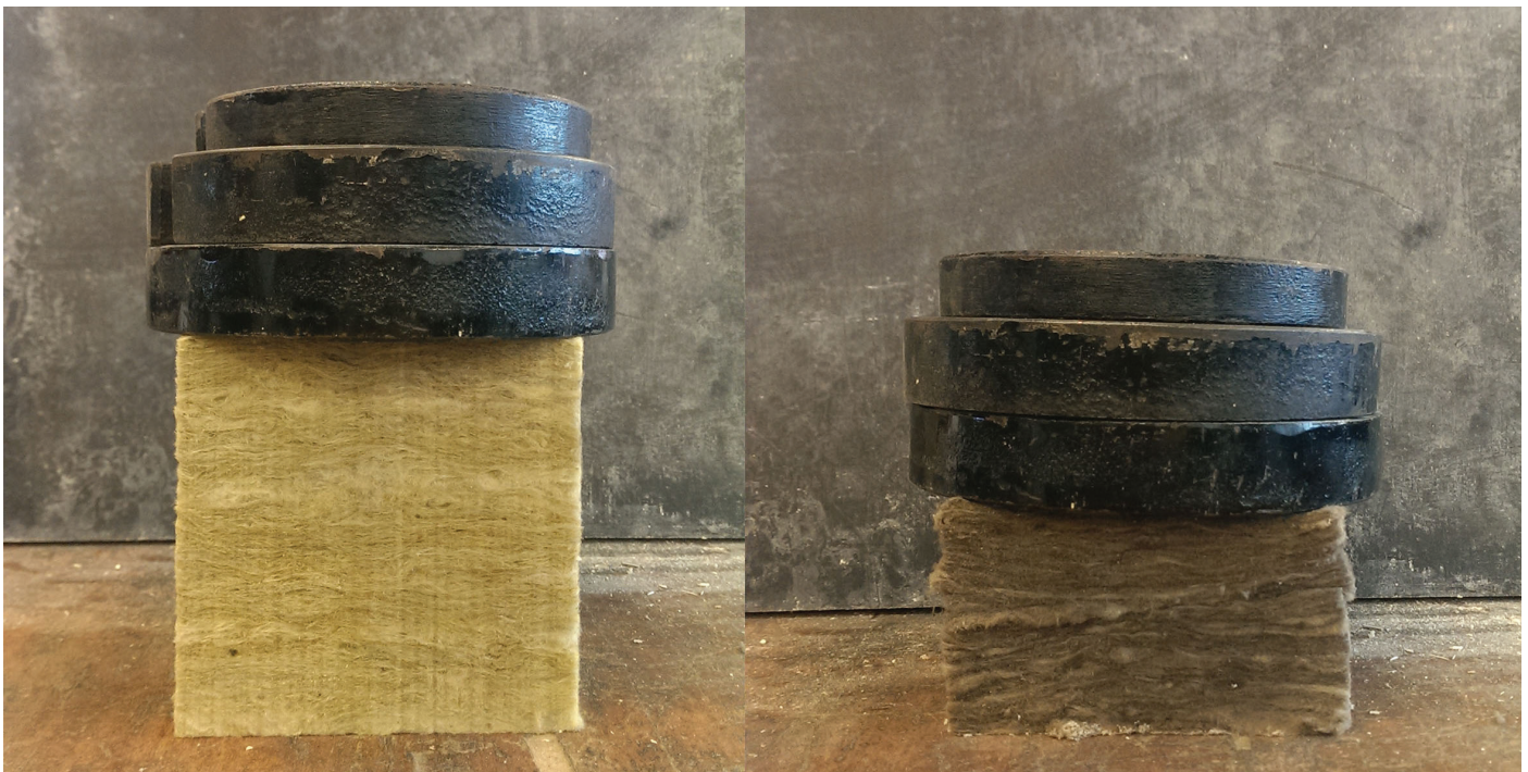
Figure 44 - loss of structural strength, load : 5KG
