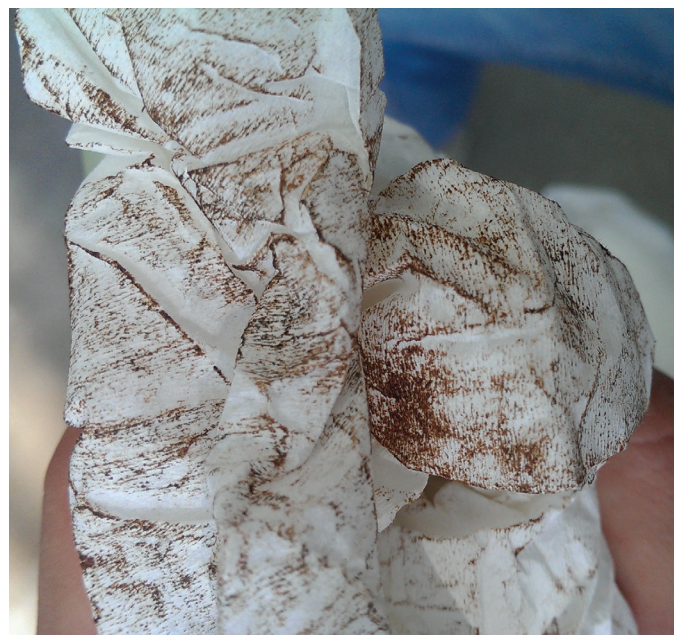
Figure 37 - Colour of the PIR effluents condensate
