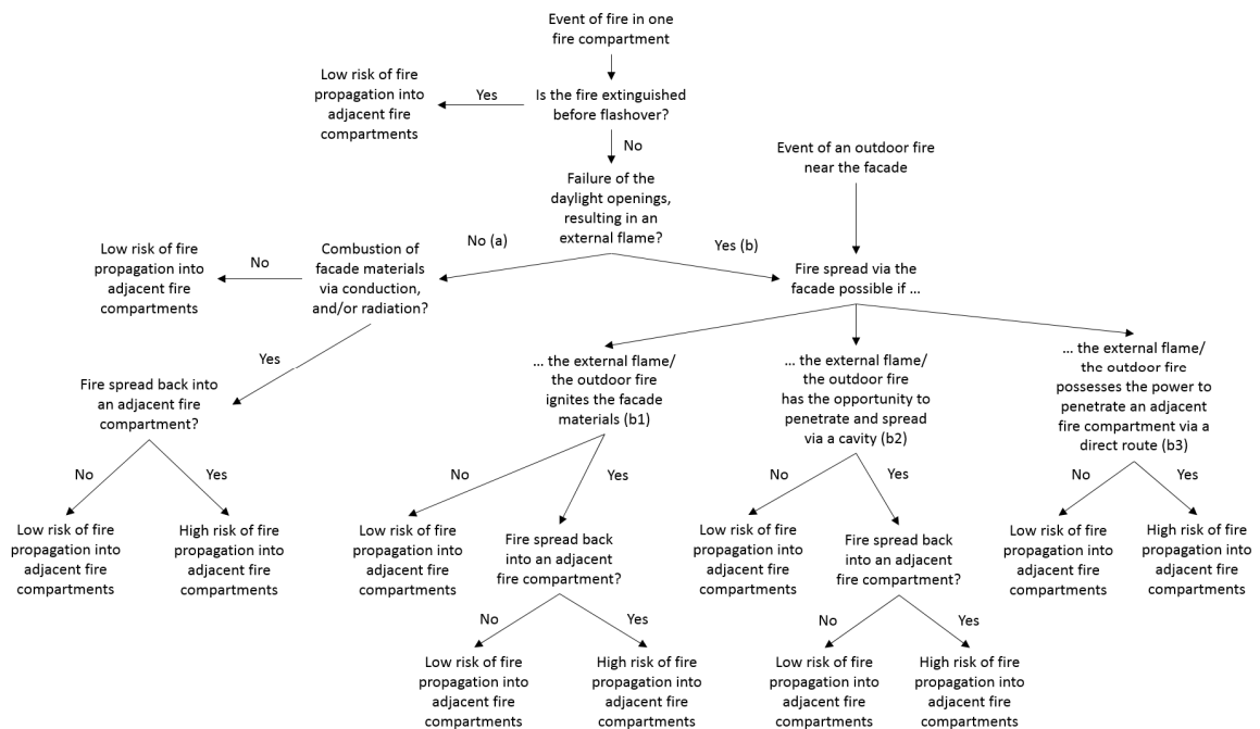
Figure 1. Failure risk tree for compartment fires
