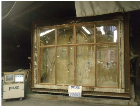
Figure 9: experimental setup double glazing
