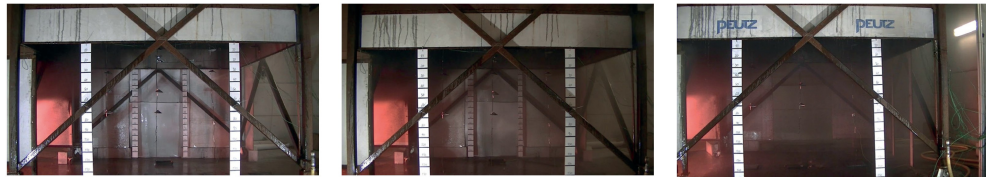
Figure 7. Smoke logging, water flowrate 56, 71 and 93 l/min
