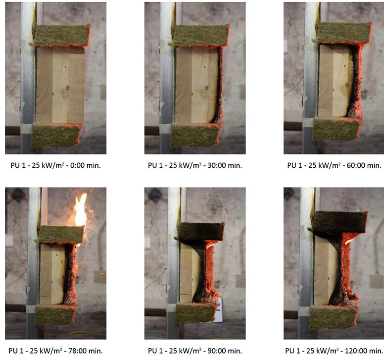
Figure 40. Time-lapse PU 1. 25 \text{ kW/m}^2 for 120 min. Re-ignition at minute 76.
