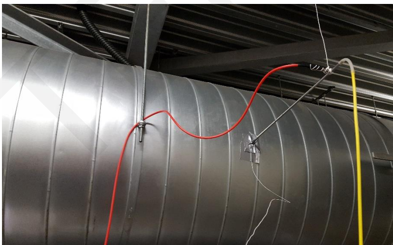
Figure 6 - Measurement set-up reference point (left), manometer (right)
