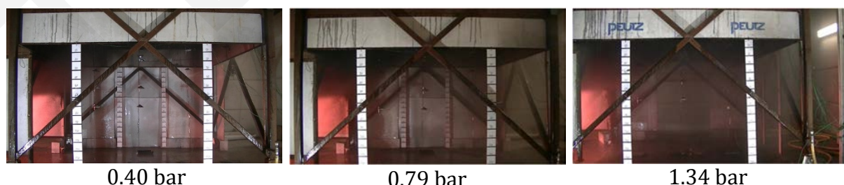
Figure 38 - Smoke logging during sprinkler experiments (multiple operating pressures)
