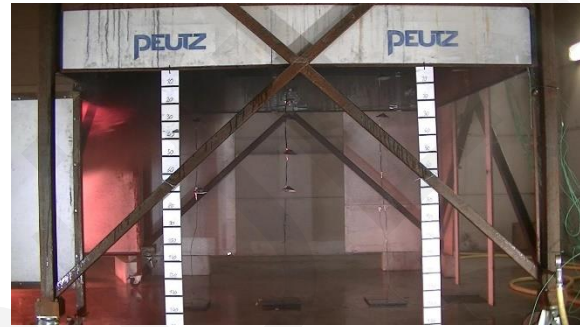
Figure 16 - Snapshot smoke layer height SH4 after 133 seconds, sprinkler active for 10 seconds
