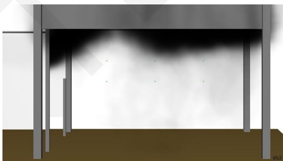
Figure 5 - Snapshot smoke layer height in FDS SH1 after 126 seconds, sprinkler active for 30 seconds
