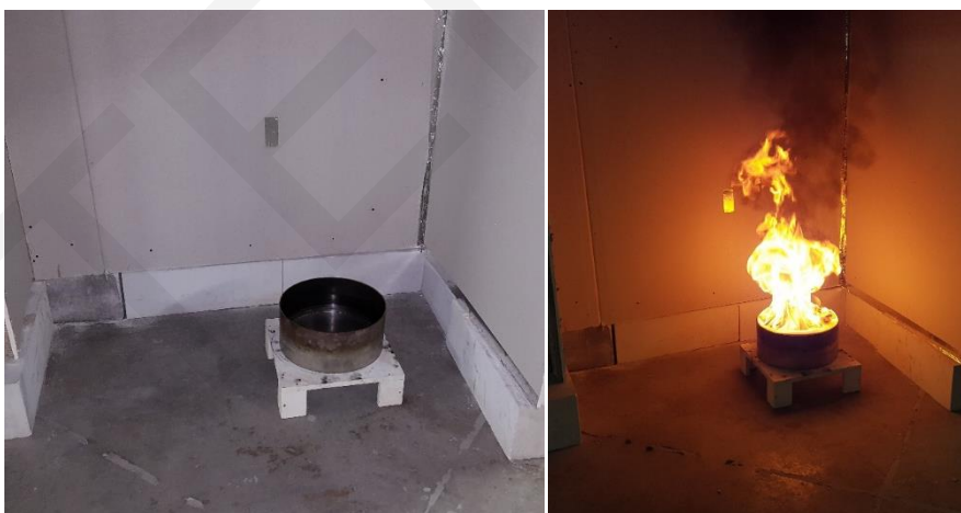
Figure 2 - (left) set-up repetition SBI heptane/toluene calibration, (right) burning of heptane/toluene
