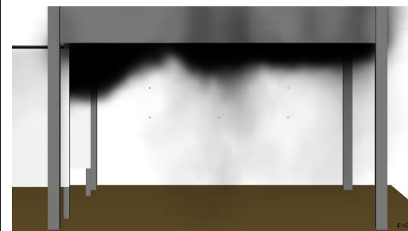
Figure 6 - Snapshot smoke layer height in FDS SHT1 after 184 seconds, sprinkler active for 30 seconds
