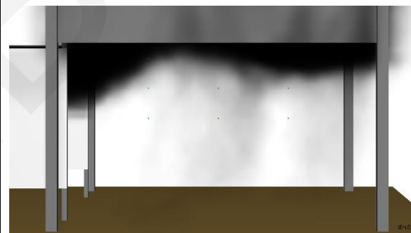
Figure 4 - Snapshot smoke layer height in FDS SHT1 after 164 seconds, sprinkler active for 10 seconds
