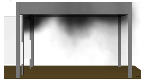
Figure 12 - Snapshot smoke layer height in FDS SH3 after 150 seconds, sprinkler active for 30 seconds
