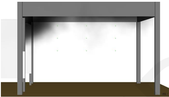
Figure 9 - Snapshot smoke layer height in FDS SH2 after 128 seconds, sprinkler active for 10 seconds
