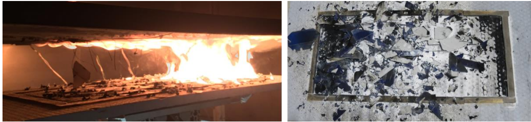
Figure 41 Debris from combustible panel on the sample set-up
