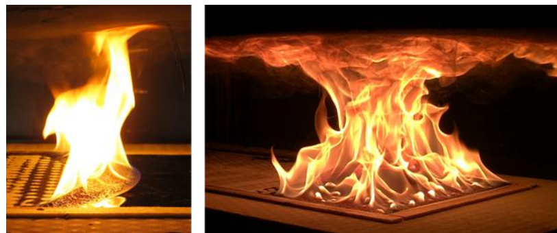
Figure 17 Surface bubbling in the growth phase (left) and the accelerated phase (right)
